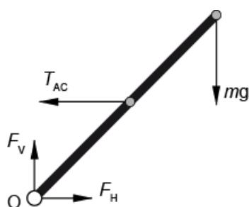
b)  $\sum M(0) = 0 \rightarrow mg \cdot 2L = T_{AC}L \rightarrow T_{AC} = 3923 \text{ N}$
